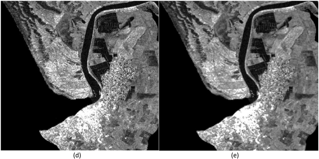
Figure 10. Visual representation of: (a) SAR Sentinel 1 GRD VV Polarization before despeckling, (b) Sentinel 2 RGB bands used as guided image, (c) SAR Sentinel 1 GRD VV Polarization after despeckling, zoomed region of SAR data: (d) before and (e) after despeckling.
