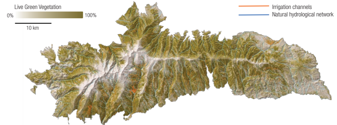
Distribution of the natural hydrological network in Sierra Nevada (blue) in comparison with the network of ancient irrigation channels (orange). The background image shows photosynthetically active vegetation (green), bare soil and snow (both light coloured). USGS/NASA Landsat 5 TM 2011-06-19. Irrigation channel data courtesy of EU F7 MEMOLA project.
