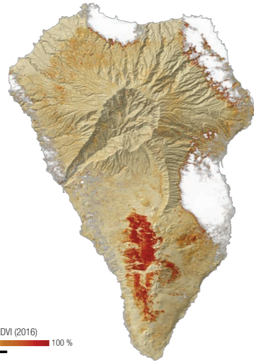
Decline in NDVI product derived from Sentinel-2A (2016) which shows the loss of vegetated area in the southern part of La Palma between July and August 2016 due to a fire episode. Clouds, which continuously form due to trade winds, cover the white areas on the map. Produced from ESA remote sensing data (Sentinel-2A). LiDAR based Digital Elevation Model processed by CESBIO for ECOPOTENTIAL. Data processing by UBT for ECOPOTENTIAL.
