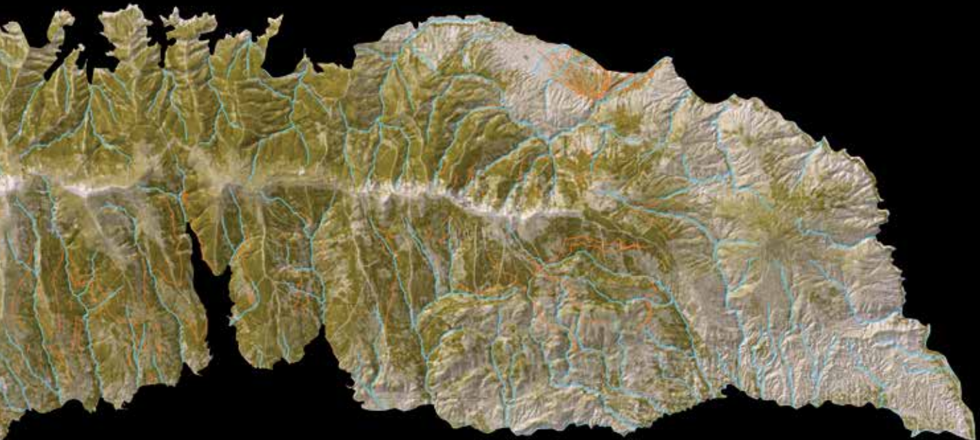
Distribution of the natural hydrological network in Sierra Nevada (blue) in comparison with the network of ancient irrigation channels (orange). The background image shows photosynthetically active vegetation (green), bare soil and snow (both light coloured). USGS/NASA Landsat 5 TM 2011-06-19. Irrigation channel data courtesy of EU F7 MEMOLA project.
