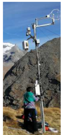
Eddy Covariace tower equipped for CO 2 fluxes and for micrometeorological monitoring
